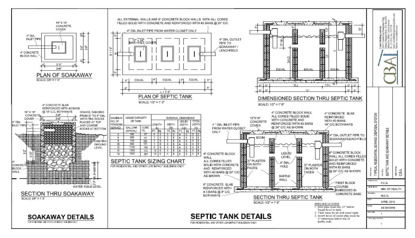
Figure 10: Septic Tank and Soak-a-way Details for Residential and Low-Impact Buildings
