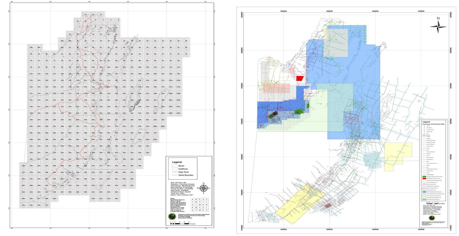
Figure 21: (a) Base map of the Block and Sub-block System used to manage Exploration in Belize. (b) Map of current and historical geophysical surveys and wells drilled in Belize
