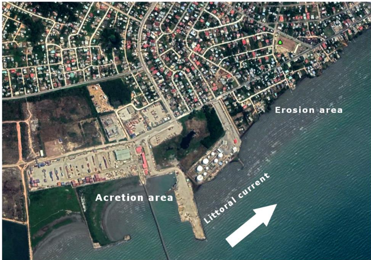
Figure 28 Erosion and accretion zones due to the construction of the Port of Belize
